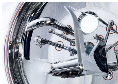
Scraper knife over the entire basket height, feed and wash pipe
