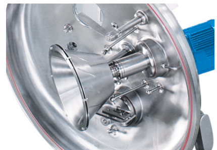
Scraper knife with vertical movement, feed and wash disk
