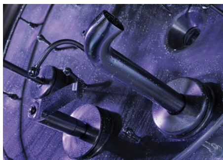
Riboflavin Test - after CIP
