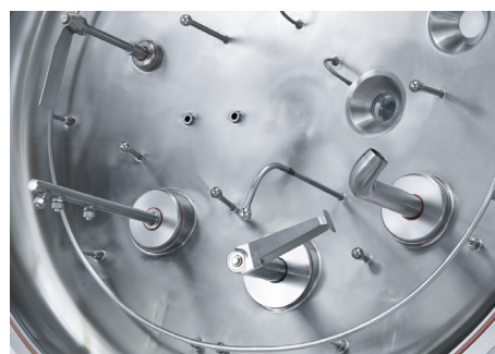
Feed and wash pipe, cake loosening device
